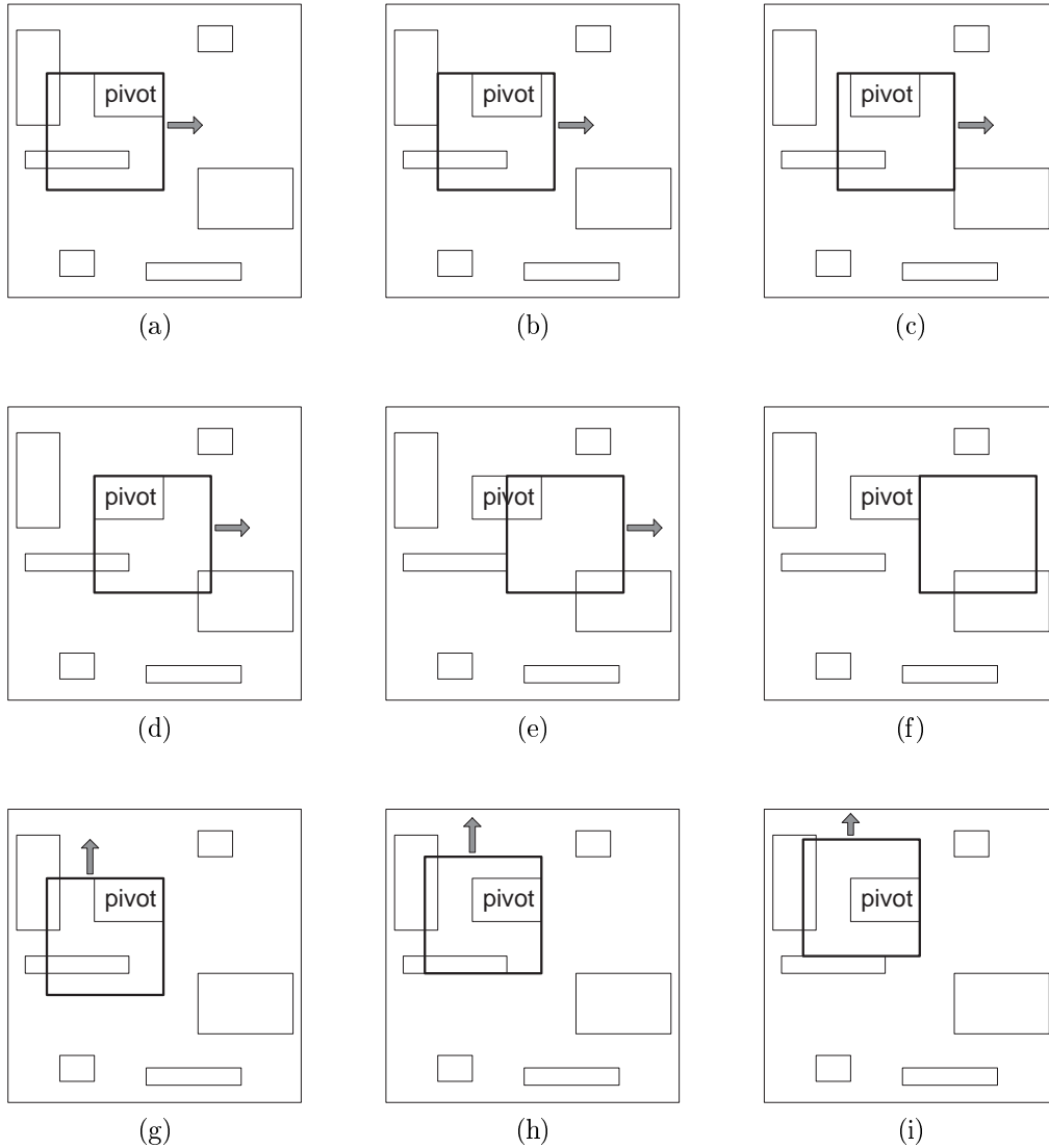
Figure 6: ALG2 starts a window abutting a pivot rectangle (a) and slides the window to the right, stopping at each edge that intersects its perimeter (b), until the pivot abuts the opposite side of the window, on the outside (f). Other combinations of the pivot-window orientations are then explored (g-i). This process is repeated for every rectangle, using each as a pivot in turn.
